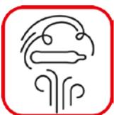
For a quick release of the E-Bulb, the placement of the bulb should be located in the potentially resulting airflow of the convection.
