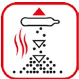
In principal the E-Bulb should be placed as high as possible in the housing. The extinguishing medium NOVEC is heavier than air and thus automatically sinks to the bottom of the housing. In addition, the warm air rises in a fire. The E-Bulb should therefore be placed in thermals created by the hot air flow. This allows a faster activation.
