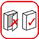
In the best case, the housing is completely closed. If, due to ventilation slits or design requirements, there is no completely enclosed room available, the more closed the electronic housing the better and more likely it is to be able to extinguish the fire.
