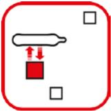
To increase the extinguishing effectiveness, it helps to identify the possible hotspots in order to place the E-Bulb optimally. The closer the E-Bulb is placed to the potential source of fire, the better. However, make sure that in case of a fire the convection of the air reaches the E-Bulb. Attention is especially required in "corners".
