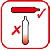
To activate the E-Bulb it requires a complete warming of the E-Bulb. A horizontal installation position is often recommended.
